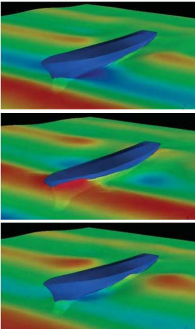
The above images show a transient ship hull-wave interaction calculation that was performed using ANSYS CFX software and custom FORTRAN code. ANSYS CFX determines the forces acting on the boat, FORTRAN relates the forces to the hull motion.
