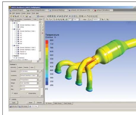
Specialized interfaces in the ANSYS CFX product provide direct access to many of the parameters, all within the ANSYS Workbench environment.
