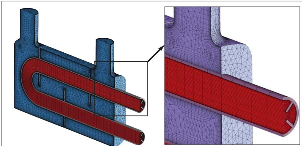
ANSYS CFX software allows any combination of meshes to be used. This hybrid mesh allows for the use of automated meshing approaches where possible, but maintains excellent near-wall mesh spacing to give good resolution of boundary layers. For this example, extruded hex and hex-prism meshes were used for the pipe solid walls and fluid interior, while the shell side mesh is a combination of prism and tet elements.
